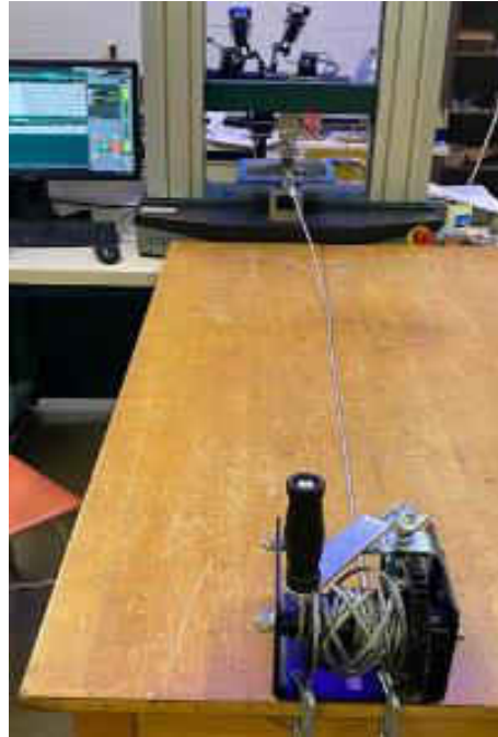
Figure 72 Winch and DIC Setup
