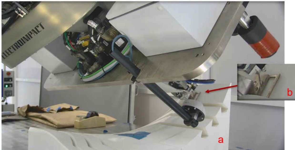
Figure 6 Presser Foot Collision: (a) 3D Printed Surface to hold Fabric, (b) Presser foot collision with surface without fabric
