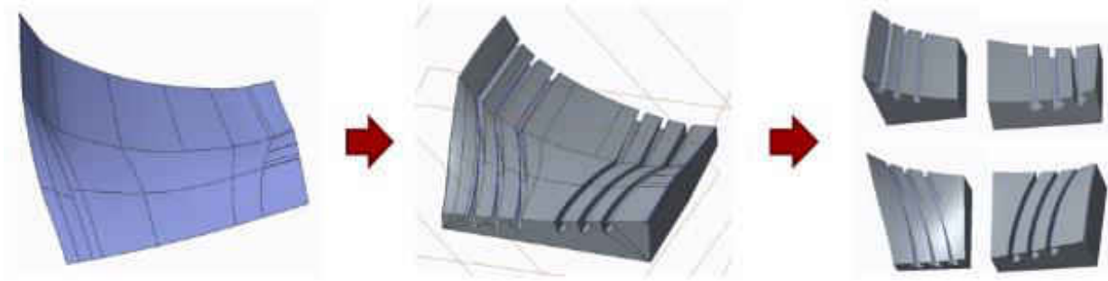
Figure 5 Wind Tunnel Blade Model Created Using CREO Parametric
